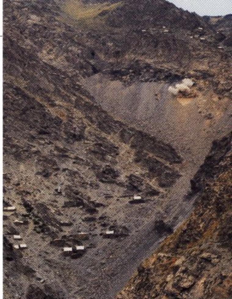
Figure 6. Blasting is common in all of the Panjshir Valley emerald mines. At the Khenj mine shown here, a smoke cloud can be seen toward the top of the diggings, the result of blasting in the mine shaft. Note also the large amount of waste material dumped from the mine. Photo by Gary Bowersox.
