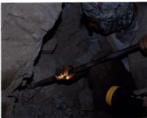
Figure 9. Picks and crowbars are also used in the mine to remove loosened wallrock. Photo by Gary Bowersox.
